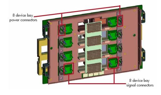
Figure 9. Diagram of the HP BladeSystem c3000 signal midplane
